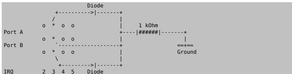
The cathodes of the diodes are connected to a common point, together with a 1 kOhm pull-down resistor. It is essential to connect the resistor to ground to avoid floating of the IRQ line on the bus.
